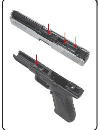
locking stepped portion of the parrel hood. Put one drop in the slide up front sight down to let it run the length of the slide rails. Use a small dab of molybdenum grease on the surfaces where surfaces where there is metal-on-metal contact, like the firing pin safety punger and striker heal.
